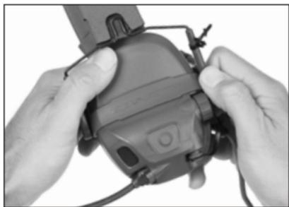
3. Find / hold center point of ear-to-ear cable. Fold the middle cable retention tab over center point of cable.
