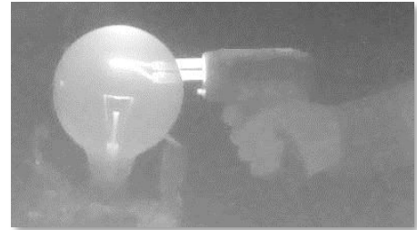
MWIR image using Phoenix Core (3-5 \mu\text{m} ) The filament and Soldering Iron are visible
