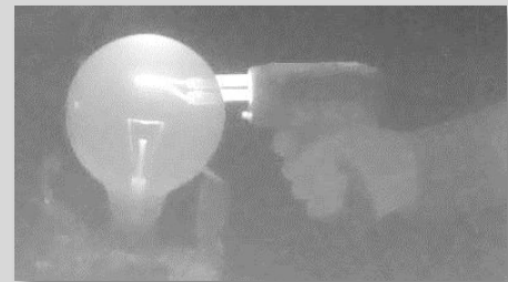
MWIR image using Phoenix Core (3-5µm) The filament and Soldering Iron are visible
