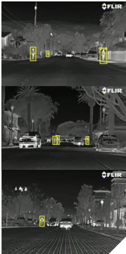
PathfindIR II with onboard analytics
